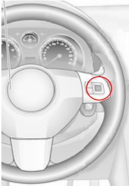
The desired data is shown on the display that normally shows the odometer and the daily counter.
